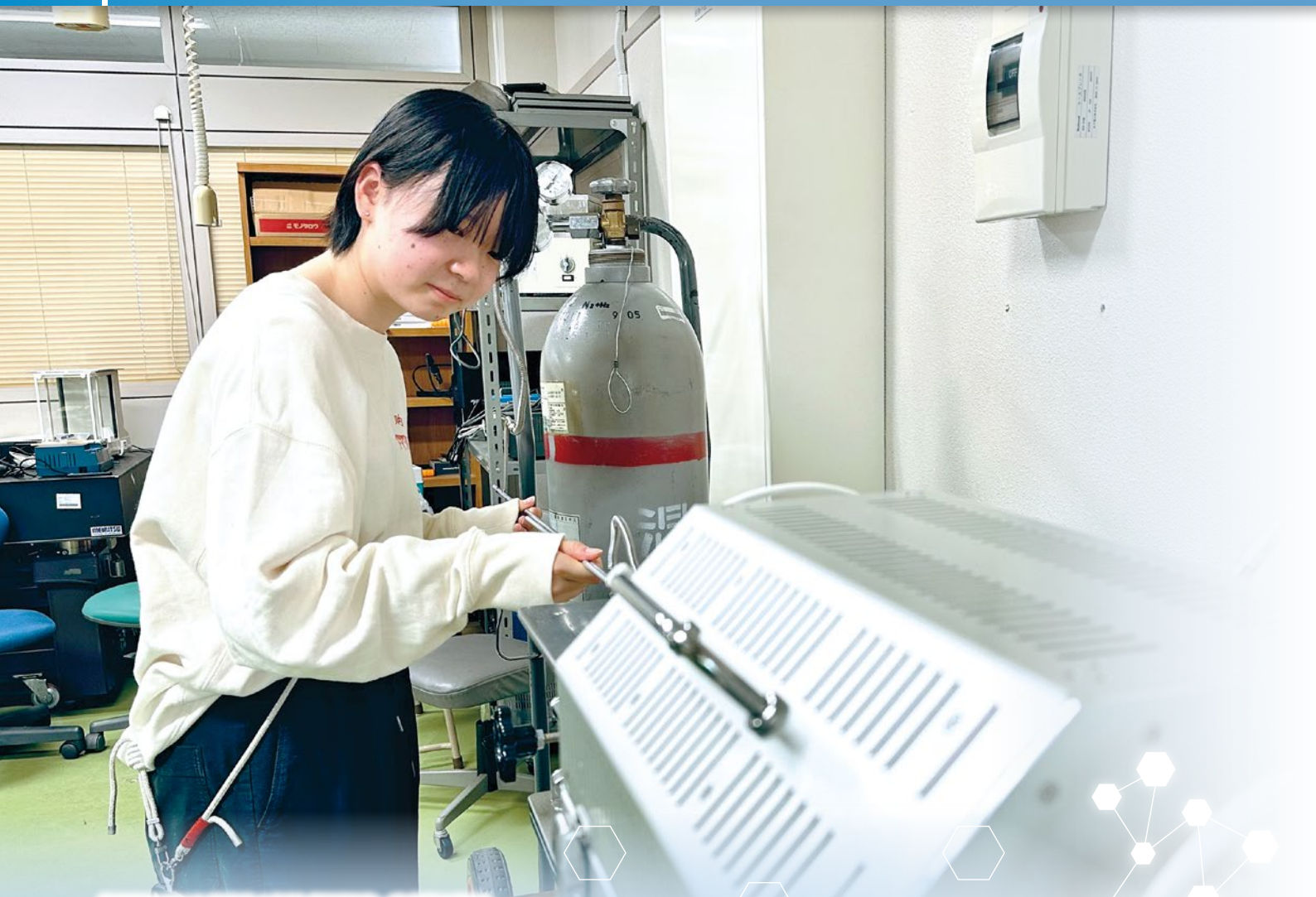
管状炉を用いた蛍光体の作製（特別研究・専攻科1学年） Fabrication of phosphor by tube furnace (Thesis work, advanced course 1st grade)
