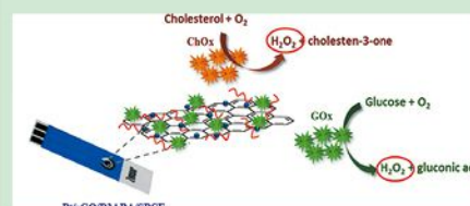
Fig.2 Developed glucose and cholesterol biosensors [5].
