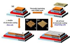
Fig. 1 Developed OSCs with plasmonic grating nanostructure [3].
