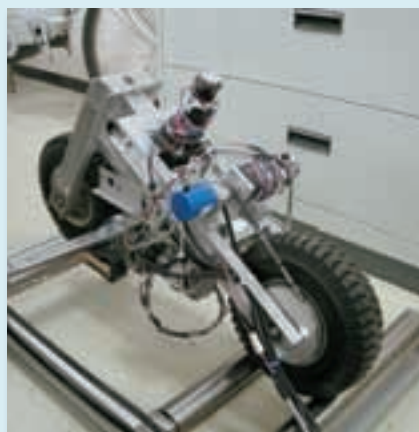
自立走行二輪車の安定化制御 Stabilizing Control of Self-Sustaining Two-wheeled Vehicle
