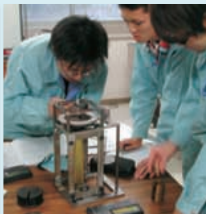
ゴム棒の静的ねじり試験(機械工学実験実習・3学年) Static torsion test on rubber rod (Experiments in Mechanical Engineering, 3rd grade)
