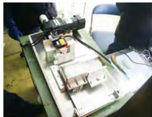
貯雪の強度試験 Strength Test of the Stored Snow
