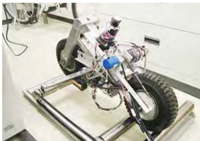
自立走行二輪車の安定化制御 Stabilizing Control of Self-Sustaining Two-wheeled Vehicle
