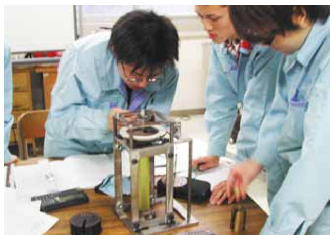
ゴム棒の静的ねじり試験（機械工学実験実習・3学年） Static torsion test on rubber rod (Experiments in Mechanical Engineering, 3rd grade)
