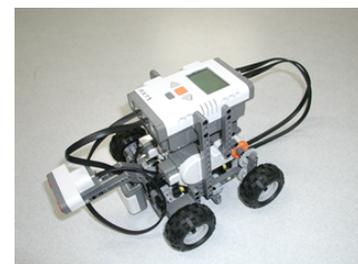
Fig.2 Line trace robot
